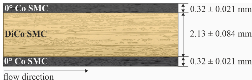
Fig. 2. Schematics of the cross section of [Co/DiCo/Co] specimens. The longitudinal direction of the specimens corresponds to the flow direction of DiCo SMC and the direction of the continuous fibers.
