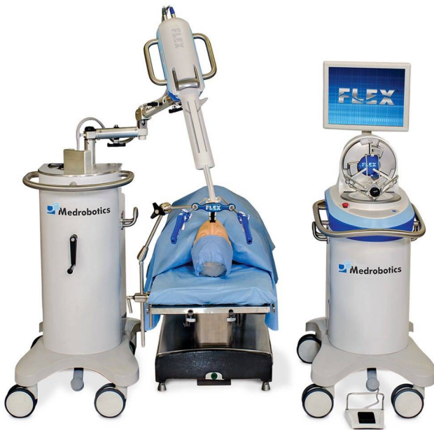
Fig. 1 Flex system setup featuring a HD-monitor control unit with a joystick for basic positioning and forwarding of the endoscope, and a base module, where the endoscope attaches. The endoscope is driven computer assisted by joystick, while the flexible instruments are manipulated independently by the hand of the surgeon
