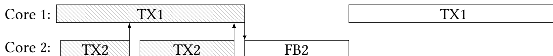
Figure 5.2: When transaction 2 (TX2) reaches its limit of attempts to commit it is executed in fallback mode. After the fallback execution (FB2) finished, Transaction 1 (TX1) is re-executed and can try again to commit. This mechanism can lead to serialization, preventing parallelism, since FB2 has to be executed exclusively preventing transaction 1 to be executed. Since the original scenario (see Figure 5.1) prevented any progress, it still makes sense to utilize the fallback path.
