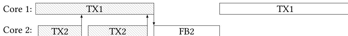
Figure 5.2: When transaction 2 (TX2) reaches its limit of attempts to commit it is executed in fallback mode. After the fallback execution (FB2) finished, Transaction 1 (TX1) is re-executed and can try again to commit. This mechanism can lead to serialization, preventing parallelism, since FB2 has to be executed exclusively preventing transaction 1 to be executed. Since the original scenario (see Figure 5.1) prevented any progress, it still makes sense to utilize the fallback path.
