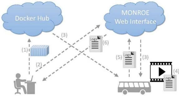
Fig. 2: Procedure for scheduling an experiment in the MONROE testbed in six steps.
