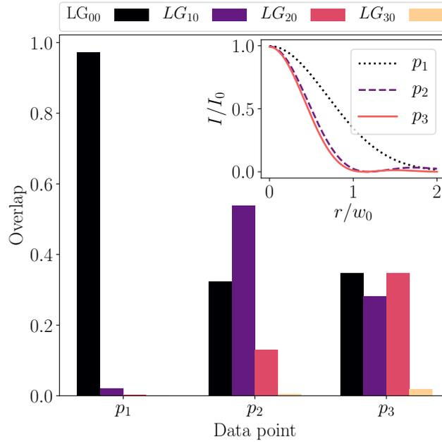
Figure 5: The overlap of different LG modes with the total cavity field at the three points, in  $(\omega, \Lambda)$  space, marked by green crosses in Fig. 4 (b):  $p_1 = (0.04, 0.77)$ ,  $p_2 = (0.42, 0.49)$ ,  $p_3 = (0.62, 0.37)$ . The inset shows the resulting total intensity profiles of the modes in real space, which are radially symmetric. The intensity  $I$  is defined as the absolute square of the mode function.
