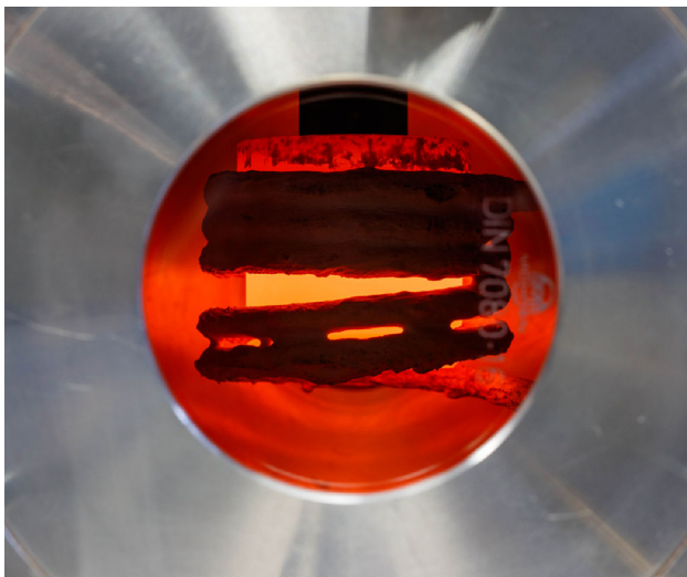
Figure 5. Inductively heated graphite crucible. View through the sight glass of the Induction Analysis Furnace (IAF).
