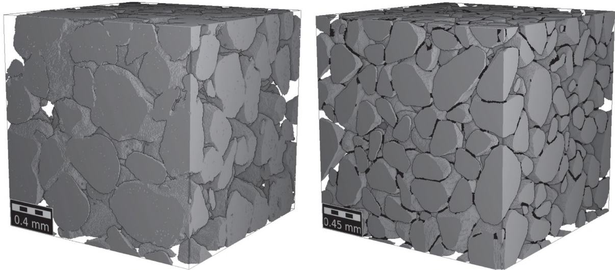
(a) 1/64th of a \mu CT image, with 59.04% sand and binder (cannot be separated) (b) Computer-generated volume element with 58.55% sand (grey) and 1.5% binder (black)
