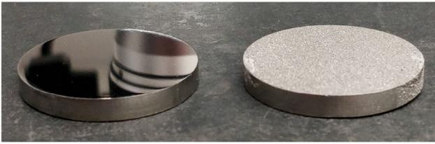
**Figure 5. Mirror-finish-polished specimen (left) and sodium silicate binder sprinkled specimen after hardening (right).**
