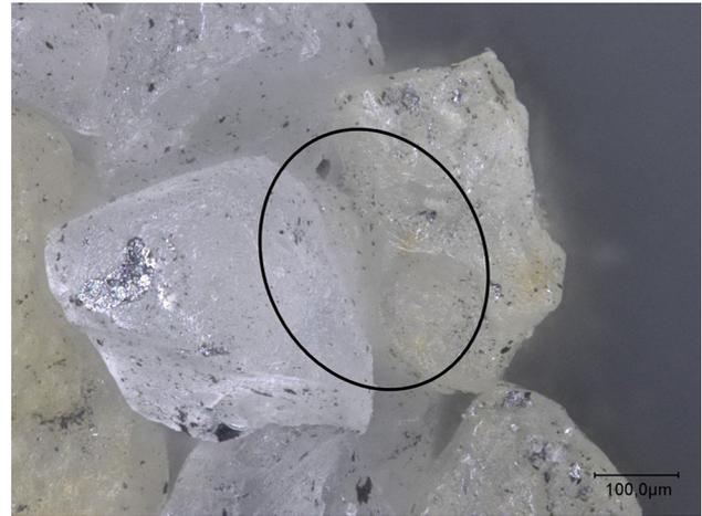
**Figure 4. Binder bridge under the microscope.**
