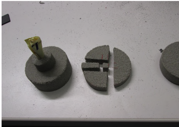
(a) Cylinder specimen, sawn into pieces.
