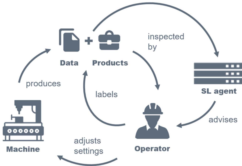
Figure 2. Assisted production using an agent trained with supervised learning (SL) during operation.
