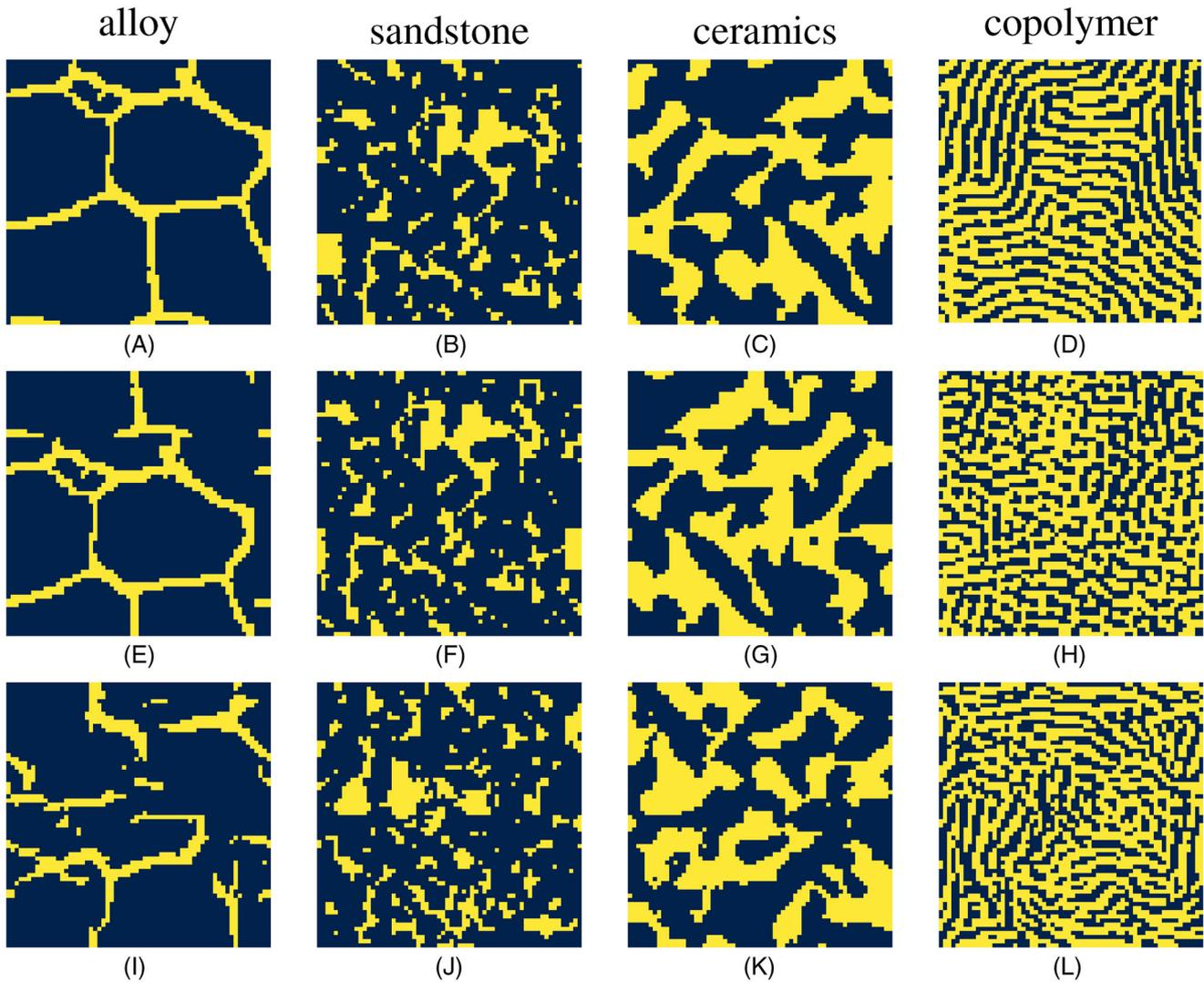
**FIGURE 4** Comparative overview of the reconstruction properties using a spatial correlation function as descriptor and a scattering descriptor. The figure reads as follows: (A)–(D) are original microstructure samples of pixel size  $64 \times 64$  taken from [19], (E)–(H) are reconstructions using a spatial correlation function and (I)–(L) are reconstructions using the above introduced scattering descriptor.
