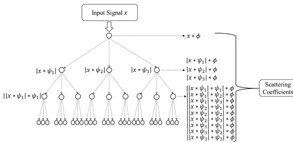
**FIGURE 3** Computational Structure of the Scattering Transformation.  $\psi$  denotes the wavelet kernel and  $\phi$  the gaussian kernel. In this example three different wavelets are used for the convolution, which gives  $3^i$  nodes for layer  $i$ . The illustration was created by Varun Khemani et al. [25] and is used, without modifications made by the author, under the Creative Commons BY license.
