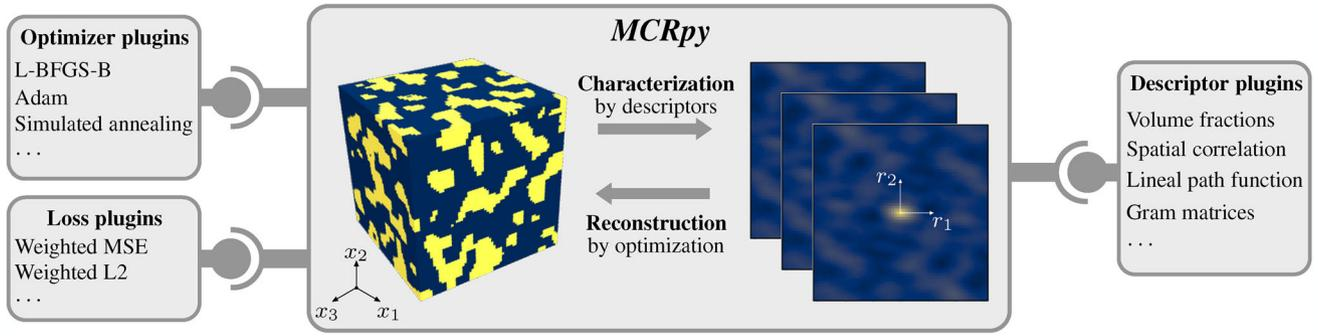
**FIGURE 1** Structural overview of MCRpy: microstructures can be characterized and reconstructed, whereas the preferred optimizer, loss function and descriptor are provided as plug ins. The illustration was created by Paul Seibert et al. [21] and is used, without modifications made by the author, under the Creative Commons BY license.
