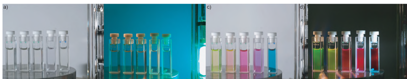
Figure 1. Irradiation of stirred solutions of Rhodamines NN in ethanol (from left to right in each picture: 2a-H , 2b-H , 2c-CO 2 Et , 2d-CO 2 Et , and 2e-F ) with UV light from a middle-pressure mercury lamp (150 W) equipped with Pyrex filter ( \lambda > 330 nm) provides highly fluorescent dyes of five principal colors. a) Starting solutions are colorless or light yellow; b) the lamp is ON; c) a daylight picture taken after complete photolysis (several minutes) demonstrates the various colors of the solutions; d) a picture of the same solutions in c) taken with a torch light demonstrates the various emission colors.
