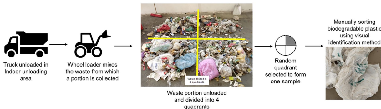
Figure 3. Sampling of residual waste in a splitting plant in Austria. Source: By Author, wheel loader icon made by Pixel perfect from www.flaticon.com.
