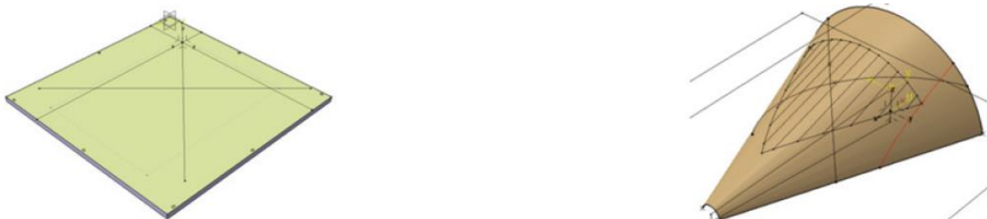
Figure 3: Illustration of the different levels of complexity. Here: complexity level 1 for a plane plate and 3 of a shell structure.
