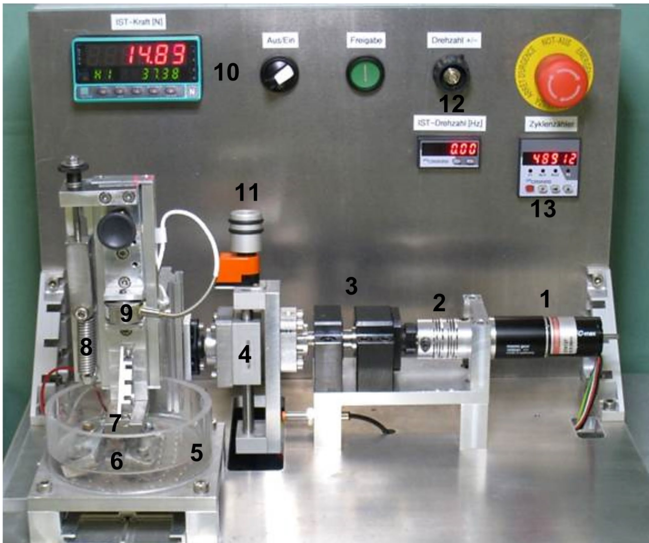
Fig. 2 Setup of the friction test stand; (1) Drive mechanism, (2) Axis of rotation, (3) Axle box, (4) Eccentric tappet, (5) Plastic tub, (6) Fixed specimen, (7) Mobile specimen, (8) Tension spring, (9) Force sensor,
