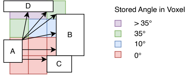
Figure 6.5: This figure illustrates how proto-relations are extracted. First, rays are cast in various directions (black arrows) starting from the anchor object (A). For each voxel that is passed by a ray, the associated ray angle is stored in the voxel. In the end only the smallest recorded angle is kept for each voxel. The ray angle is defined like with parametric relations, see also fig. 6.2.
