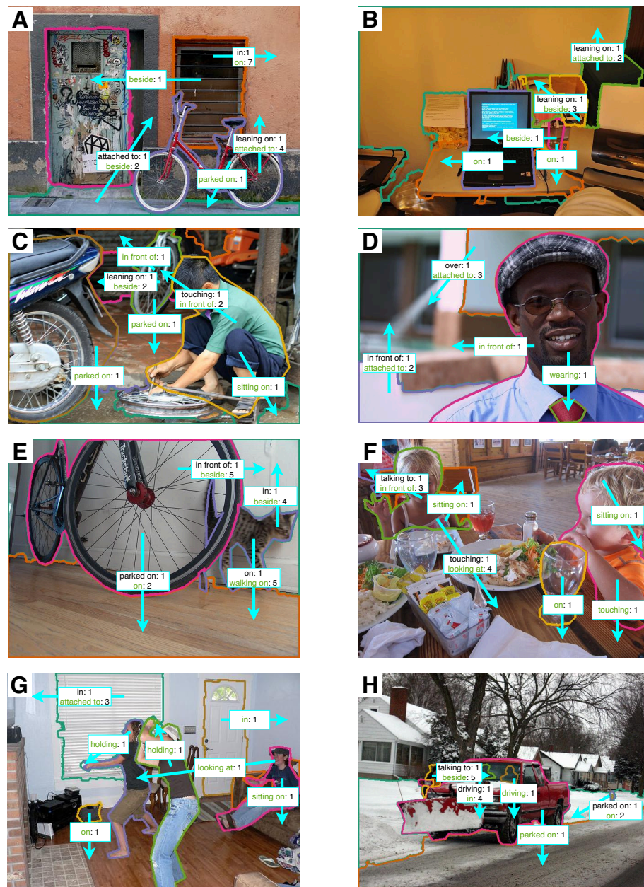
Figure 4.9: Example outputs from DSFormer. The ground truth annotation is represented by blue arrows. For each relation, DSFormer assigns a confidence score to every predicate, which can be used to rank the predicates. The ranks are displayed as numbers after a predicate name. A lower number indicates a higher confidence that the predicate fits compared to those predicates with higher ranks. The maximum possible rank is 56, corresponding to the total number of predicate classes in the PSG dataset. Green text represents the ground truth predicate label for a relation.
