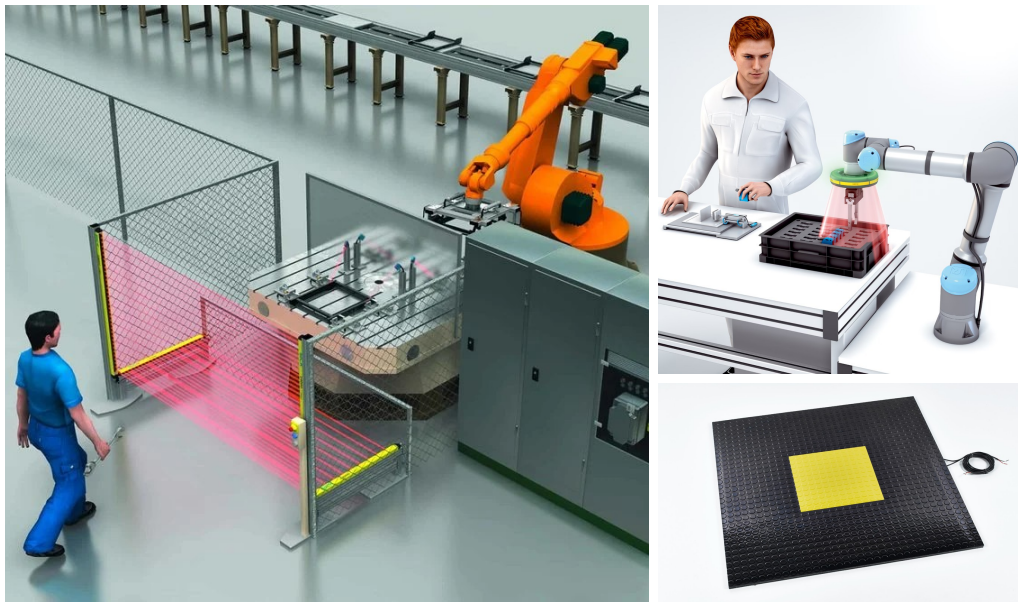
Figure 1.3. On the left, a robot system with a virtual separation by a light curtain. On the right-top, an end-of-arm-safeguard system, which protects the area around the robot end-effector. On the right-bottom, a safety floor mat, which detects when a human steps on it. Images from [204], [217], and [8].
