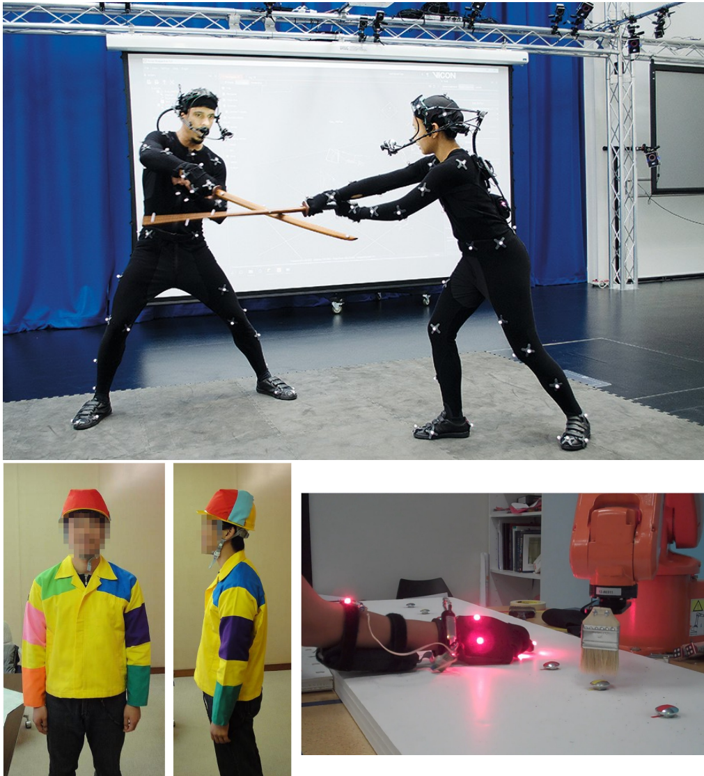
Figure 3.22. Some examples of marker-based systems. On top, a Vicon system, with the white dots serving as markers which are recorded by multiple cameras (in the background on the trusses). Image from [15]. On the bottom-left, the trackable jacket and helmet with colored markers of [226], and on the bottom-right, the active low-latency tracking glove of [138].
