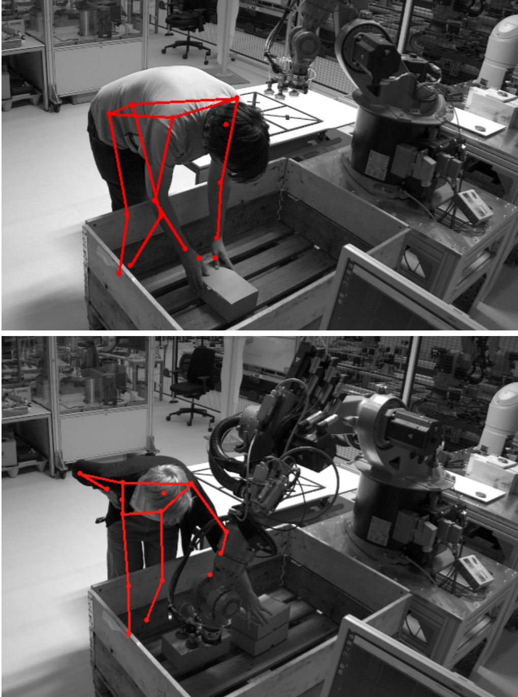
Figure 7.3. Examples in which a stop-zone would be helpful. In the images, the persons try to fetch a package themselves. They were detected by the safety system, but due to the significant occlusions and low camera coverage of this location, some joints show notable position errors. In the top image, the two red dots should be at the tips of the middle-fingers, but are substantially displaced. In the bottom image, the left hand is completely misplaced, leading to a high error between the true and detected joint position. In both cases the robot is expected to stand still. In the lower image for safety reasons, and in the upper image because the worker could feel unsafe if the robot moves while it is close and not visible. A cube-sized stop-zone covering both the pallet and the area directly in front of it, which triggers a stop if any joint is detected inside it, would allow those outliers to be ignored, because the robot will be stopped by the better detected joints already.
