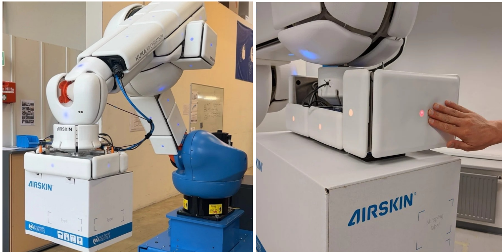
Figure 1.9. Example of additional safety cushions using the AIRSKIN system. The pads detect contact forces and also provide a soft impact protection. Images from [4].
