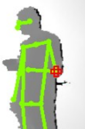
Figure 3.15. Visualization of the cross-shape used to extract the depth value for each joint in a zoom-in of the depth image. All pixels inside the cross are used to calculate the median depth distance.
