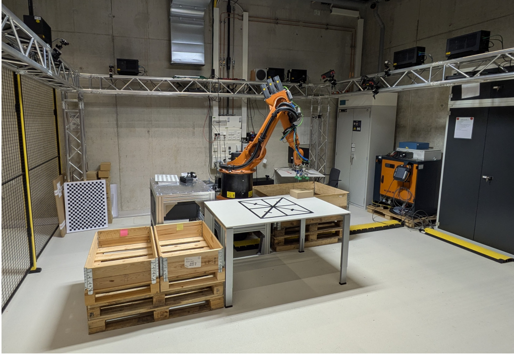
Figure 7.1. Robot setup of Tutabo-2. On top of the trusses, the new smart-camera computers are mounted.
