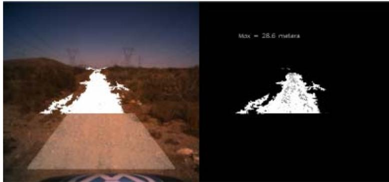
**Figure 13:** Stereo cameras can find distances to large objects. After identifying road in the left image using CART, the mean of the largest distance values produces a reasonable estimate of how far road extends in front of the car. In this example, the road extends over 28 meters ahead of the car.
