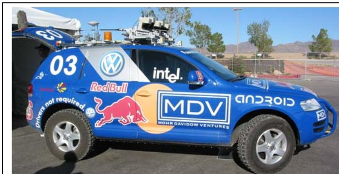
**Figure 1:** Stanford teams' VW Touareg with 5 lasers and a video camera mounted on the roof.
