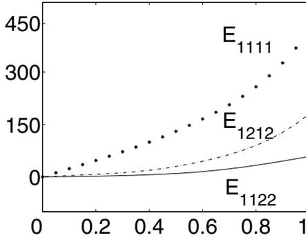
**Fig. 5.** Elastic coefficients w.r.t. density (square hole)
