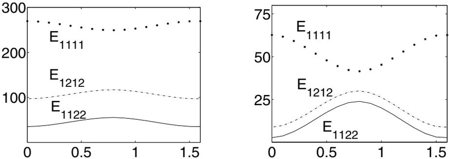
**Fig. 4.** Elastic coefficients w.r.t. to cell rotation (density  $\mu = 0.8$  and  $\mu = 0.26$ )
