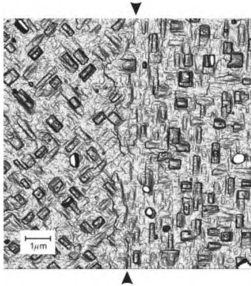
Fig. 2 – AFM image of an asymmetric 45 \pm 1^\circ bicrystalline \text{Bi}_2\text{Sr}_2\text{Ca}_1\text{Cu}_2\text{O}_{8+x} junction. The height of the growth islands is about 10 nm. The image shows that the grain boundary (indicated by the arrows) is meandering on a length scale of several hundred nanometers.
