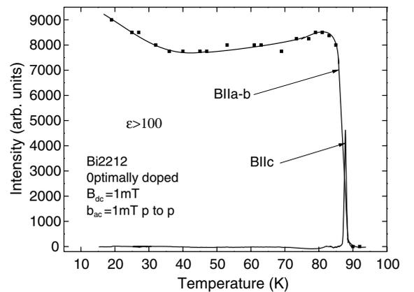
Fig. 5. Signal intensity of the Bi-2212 as a function of temperature from above  $T_c$  to 4 K for  $B\|a-b$  and  $B\|c$ . Note that for  $B\|c$  below the TAFF signal, the intensity is practically zero compared to the large intensity observed in Bi-2223, shown in Fig. 3.
