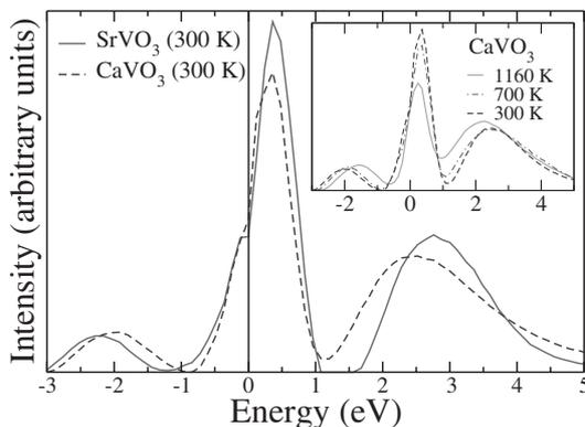
Fig. 3. LDA+DMFT(QMC) spectrum of SrVO<sub>3</sub> (solid line) and CaVO<sub>3</sub> (dashed line) calculated at  $T = 300$  K; inset: effect of temperature in the case of CaVO<sub>3</sub> (after Sekiyama *et al.*<sup>37)</sup>).
