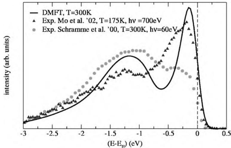
Fig. 6. Comparison of LDA+DMFT(QMC) results at  $T = 300$  K with photoemission data by Schramme *et al.*<sup>50)</sup> and Mo *et al.*<sup>48)</sup> for metallic  $V_2O_3$  (after Keller *et al.*<sup>40)</sup>).
