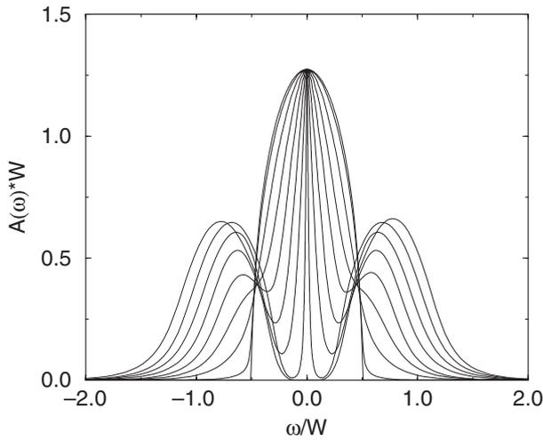
Fig. 1. Evolution of the  $T = 0$  spectral function of the one-band Hubbard model with a semi-elliptic (“Bethe”) DOS for interaction values  $U/W = 0, 0.2, 0.4, \dots, 1.6$  ( $W$ : band width) calculated with the numerical renormalization group.<sup>24)</sup> At the critical interaction  $U_{c2}/W \simeq 1.47$  the metallic solution disappears and the Mott gap opens. The “Luttinger pinning” at  $\omega = 0$  is clearly observable.
