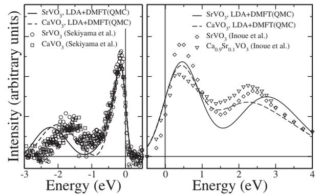
Fig. 4. Comparison of the calculated, parameter-free LDA+DMFT(QMC) spectra of SrVO<sub>3</sub> (solid line) and CaVO<sub>3</sub> (dashed line) with experiment. Left: Bulk-sensitive high-resolution PES (SrVO<sub>3</sub>: circles; CaVO<sub>3</sub>: rectangles) (after Sekiyama *et al.*<sup>37)</sup>). Right: 1s XAS for SrVO<sub>3</sub> (diamonds) and Ca<sub>0.9</sub>Sr<sub>0.1</sub>VO<sub>3</sub> (triangles).<sup>41)</sup> Horizontal line: experimental subtraction of the background intensity.
