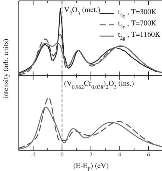
Fig. 5. LDA+DMFT(QMC) spectra for paramagnetic insulating  $(V_{0.962}Cr_{0.038})_2O_3$  and metallic  $V_2O_3$  at  $U = 5$  eV (after Keller *et al.*<sup>40</sup>).
