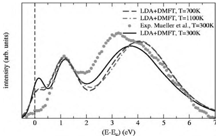
Fig. 7. Comparison of LDA+DMFT(QMC) results with X-ray absorption data by Müller *et al.*<sup>51)</sup> for metallic  $V_2O_3$  (after Keller *et al.*<sup>40)</sup>).
