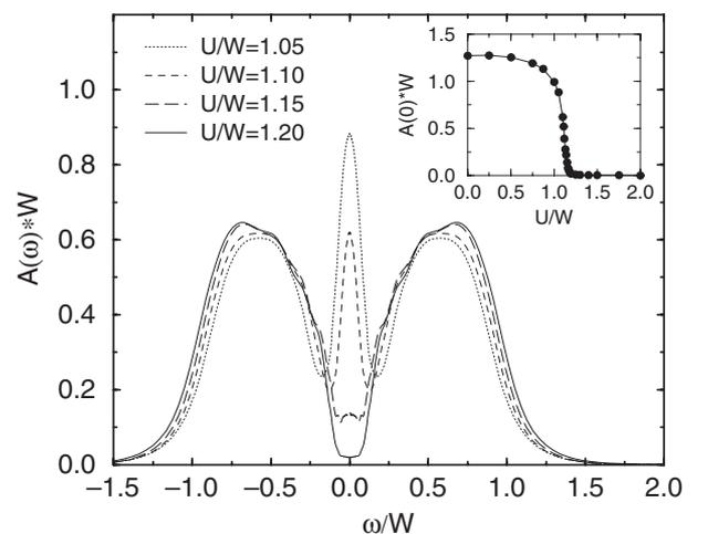
Fig. 2. Spectral function for the half-filled Hubbard model for various values of  $U$  at  $T = 0.0276W > T^*$  (in the crossover region). The crossover from the metal to the insulator occurs via a gradual suppression of the quasiparticle peak at  $\omega = 0$ . The inset shows the  $U$ -dependence of  $A(\omega = 0)$ , in particular the rapid decrease for  $U \approx 1.1W$  (after Bulla *et al.*<sup>27)</sup>).
