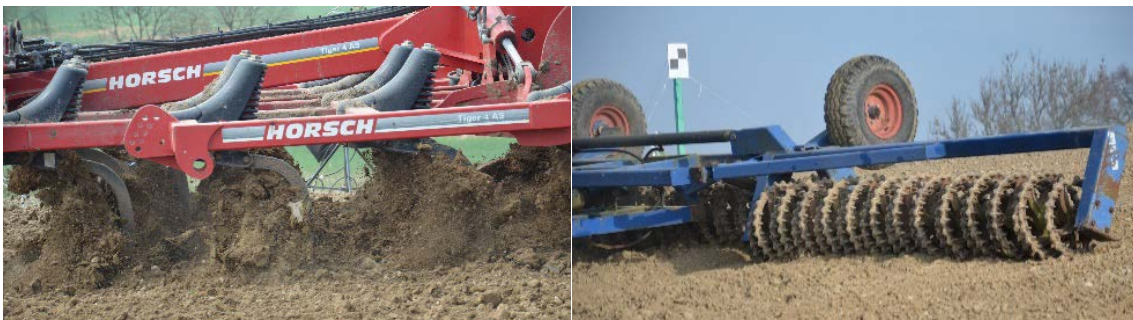
Figure 5.2: Cultivator (left) and roller (right) used during the experiment.
