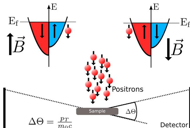
**Figure 5.** Schematic picture of spin-polarized 2D-ACAR. In electron-positron annihilation the singlet configuration is preferred for majority or minority spin electrons if the magnetization of the sample is parallel or anti-parallel to the emission direction of the positrons.
