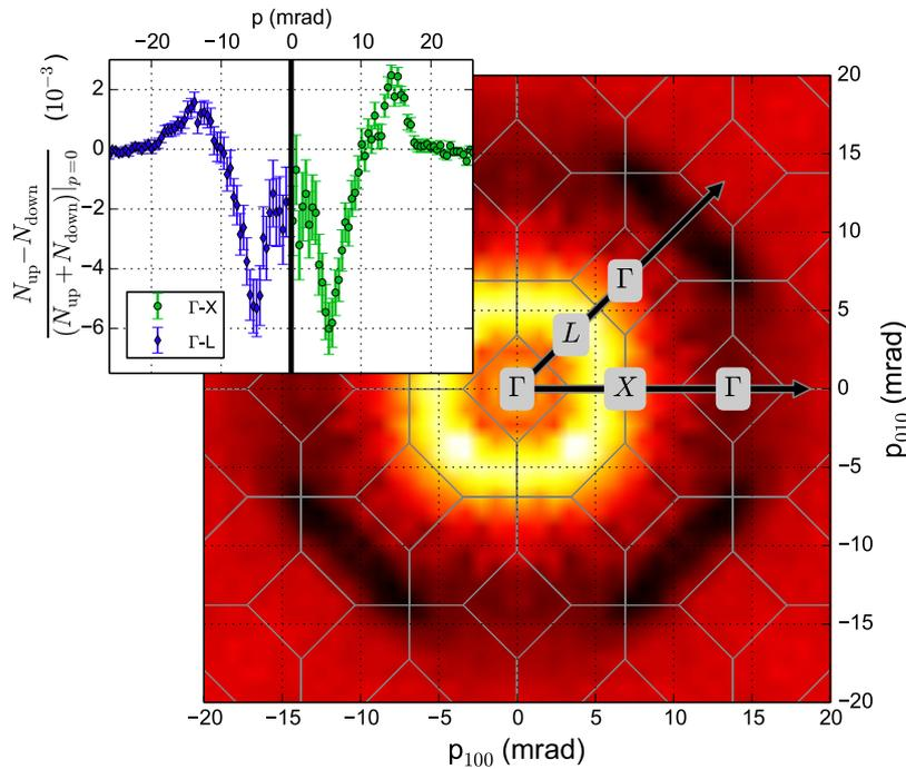
**Figure 1.** 2D-ACAR difference spectra  $\Delta N(p_x, p_y)$  obtained upon reversal of the magnetic field, with the integration along the  $[001]$  direction,  $p_x = [100]$  and  $p_y = [010]$ . The inset illustrates the anisotropy of the difference spectra between two directions in momentum space.
