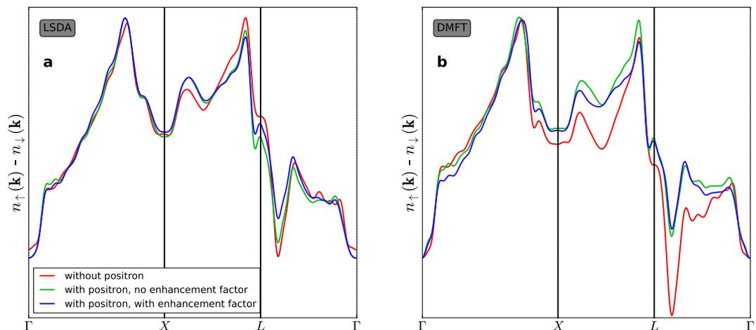
**Figure 4.** Cuts through the LCW-calculated spin-contrast along major symmetry points. The effect of the positron wave function and the combined effects of the positron wave function and the electron-positron correlations are compared with the pure electron density for calculations performed within the LSDA (a) and LSDA + DMFT (b) framework.
