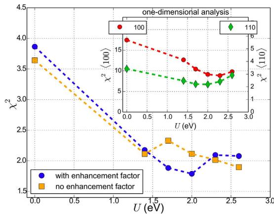
**Figure 3.** Least square fit analysis ( $\chi^2$ ) between LSDA + DMFT calculations and experimental data as a function of the Hubbard  $U$  for the 2D data. Higher  $U$  values correspond to stronger electron-electron correlations. A pronounced minimum of  $\chi^2$  is found for  $U = 2.0$  eV. The inset shows the results for the 1D data. (The dotted lines act as a guide to the eye).
