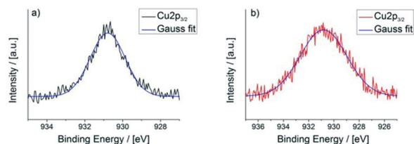
Fig. 14 Peak shape analysis of the Cu2p<sub>3/2</sub> peaks of a) CFA-9 (FWHM = 2.2 eV) and b) CFA-9 oxidized by H<sub>2</sub>O<sub>2</sub> (FWHM = 4.4 eV).
