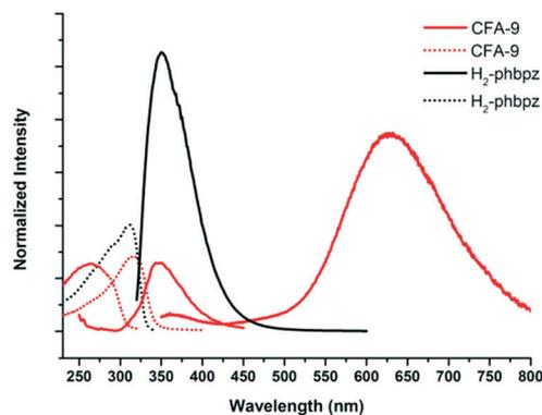
Fig. 16 Solid-state photoluminescence spectra of CFA-9 and the H<sub>2</sub>-phbpz ligand at room temperature. Dashed-lines – excitation spectra, continuous-lines – emission spectra.
