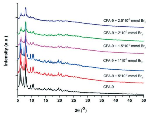
Fig. 15 XRPD measurements of CFA-9 after reaction with Br<sub>2</sub>.
