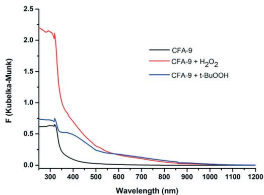
Fig. 12 UV-vis spectra of CFA-9 at room temperature. Black line – CFA-9, red – CFA-9 oxidized by H<sub>2</sub>O<sub>2</sub>, blue – CFA-9 oxidized by *t*-BuOOH.
