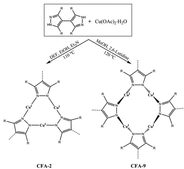
**Scheme 1** Syntheses of [Cu<sub>2</sub>(phbpz)]·2DEF·MeOH (CFA-2) and [Cu<sub>2</sub>(phbpz)]·MeOH (CFA-9) from the H<sub>2</sub>-phbpz ligand and copper(II) acetate (DEF = *N,N*-diethylformamide).
