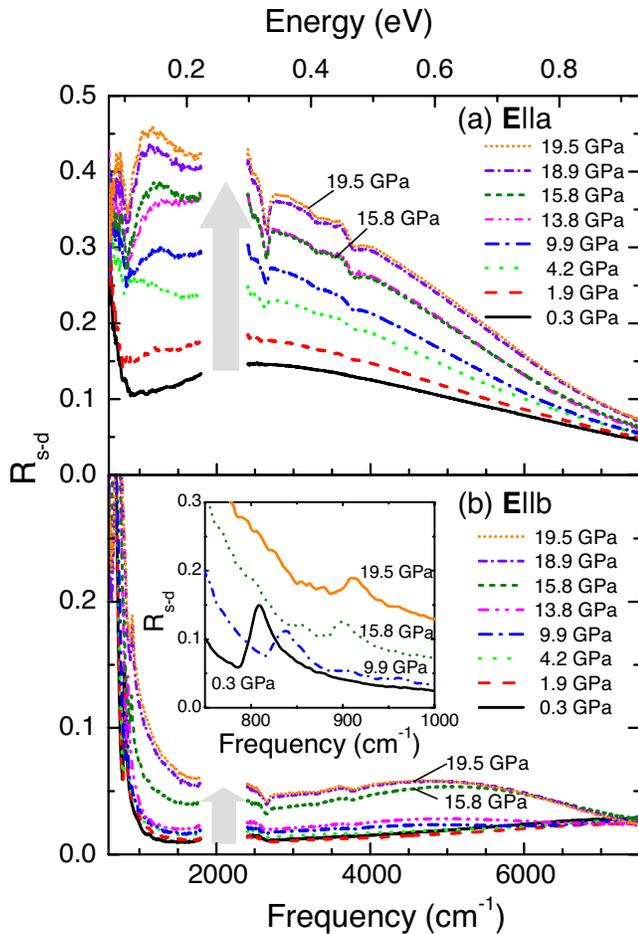
FIG. 3. (Color online) Room-temperature reflectivity spectra  $R_{s-d}$  of  $\text{LaTiO}_{3.41}$  as a function of pressure for the polarization (a)  $\mathbf{E}||a$  and (b)  $\mathbf{E}||b$ . The inset in (b) shows the low-frequency range ( $700\text{--}1000\text{ cm}^{-1}$ ) of the spectra for four pressures. The phonon at around  $800\text{ cm}^{-1}$  shifts to higher frequencies with increasing pressure. The arrows indicate the changes with increasing pressure.
