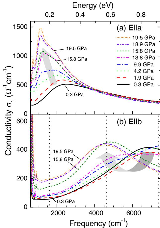
FIG. 5. (Color online) Pressure-dependent real part of the optical conductivity of  $\text{LaTiO}_{3.41}$  for (a)  $\mathbf{E}\parallel a$  and (b)  $\mathbf{E}\parallel b$  at room temperature, obtained by Drude-Lorentz fitting of the reflectivity data. The arrows indicate the changes with increasing pressure. The dotted vertical lines in (b) indicate the frequency positions analyzed in Fig. 7.
