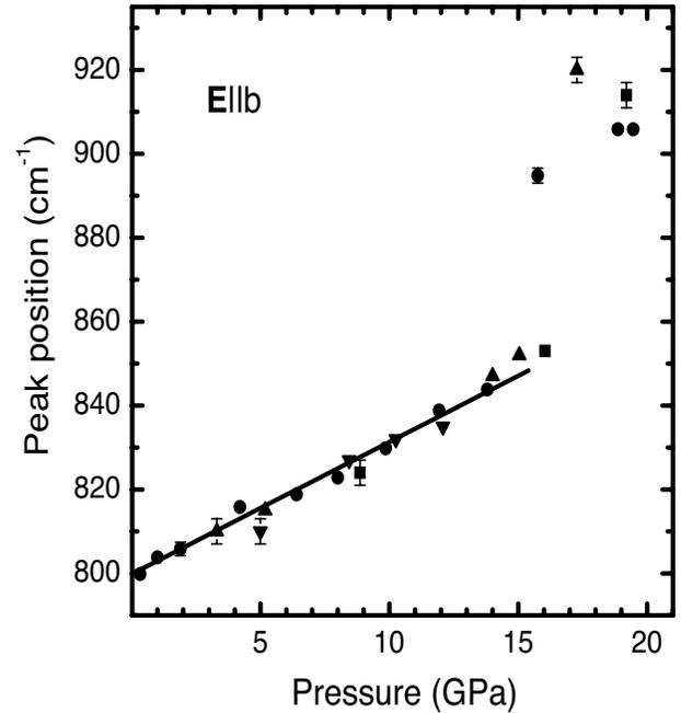
FIG. 4. Peak position of the phonon mode measured for  $\mathbf{E}||b$ . Different symbols are used for different experimental runs. Up to 14 GPa the mode hardens in a linear fashion, with a linear pressure coefficient of  $3.2\text{ cm}^{-1}/\text{GPa}$ . The line is a linear fit of the data points. At around 15 GPa an abrupt change in the frequency of the vibrational feature occurs.
