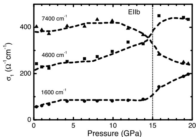
FIG. 7. Real part of the  $\mathbf{E}\parallel b$  optical conductivity at three different frequencies (1600, 4600, and 7400  $\text{cm}^{-1}$ ) as a function of pressure (extracted from Fig. 5). The dotted vertical line indicates the pressure where the structural phase transition reported earlier (Ref. 16) occurs in the present optical study. Dashed lines are guides to the eye.
