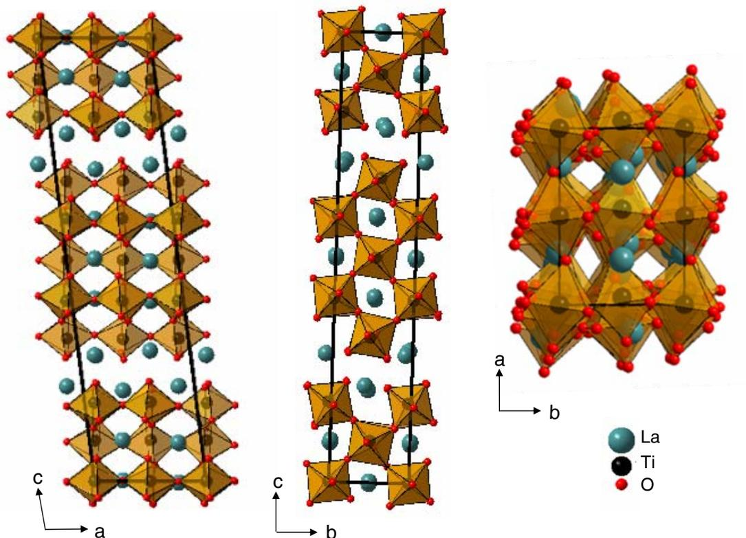
FIG. 1. (Color online) Crystal structure of  $\text{LaTiO}_{3.41}$  composed of perovskitelike slabs of vertex-sharing  $\text{TiO}_6$  octahedra, which are separated by additional oxygen layers (Ref. 15). Along the  $a$  axis the  $\text{TiO}_6$  octahedra are connected via their apical oxygen atoms forming chains.
