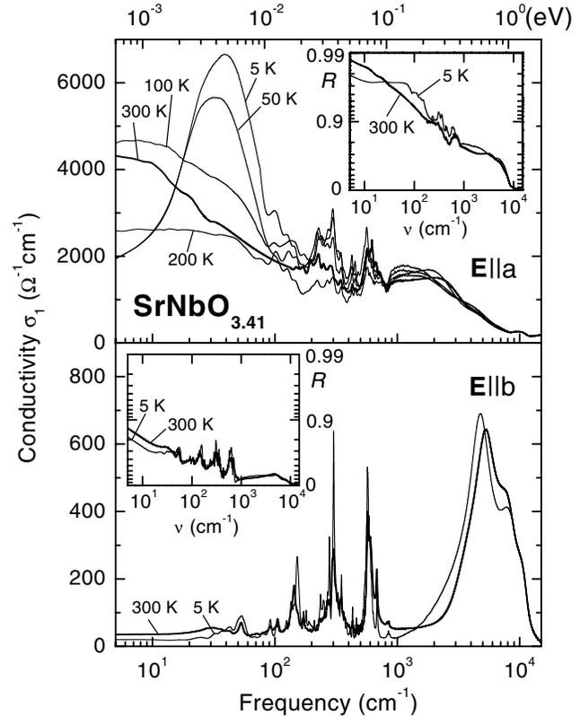
FIG. 2. Frequency dependent conductivity of  $\text{SrNbO}_{3.41}$  for different temperatures and the polarization  $\mathbf{E}$  set parallel to the  $a$  and  $b$  axes (insets: reflectivity  $R$  used for Kramers-Kronig analysis). For  $\mathbf{E}||a$ , the low-temperature peak around 40  $\text{cm}^{-1}$  indicates excitations across a gap  $2\Delta \approx 5$  meV.
