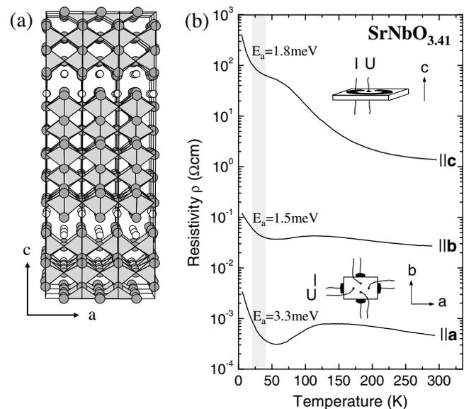
FIG. 1. (a) Projection along the  $b$  axis of the  $\text{SrNbO}_{3.4}$  crystal structure; Nb atoms are hidden within the  $\text{NbO}_6$  octahedra (light grey). White (grey) circles: Sr (O) atoms. (b) dc resistivity  $\rho$  versus temperature of  $\text{SrNbO}_{3.41}$  along the three crystal axes, with the respective measurement geometry. In the range 20–40 K (grey bar), one finds an activated behavior  $\rho \propto \exp\{E_a/k_B T\}$  with  $E_a$  as indicated.
