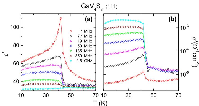
**Figure 5.** (colour online) Temperature dependence of the dielectric properties of  $\text{GaV}_4\text{S}_8$  with the electric field parallel to the crystallographic  $\langle 111 \rangle$  direction. (a) Real part of the dielectric constant between 10 and 70 K for frequencies between 1 MHz and 2.5 GHz. (b) Real part of the conductivity in a semilogarithmic plot in the same parameter range of temperatures and frequencies. In both frames, the lines are drawn to guide the eye.
