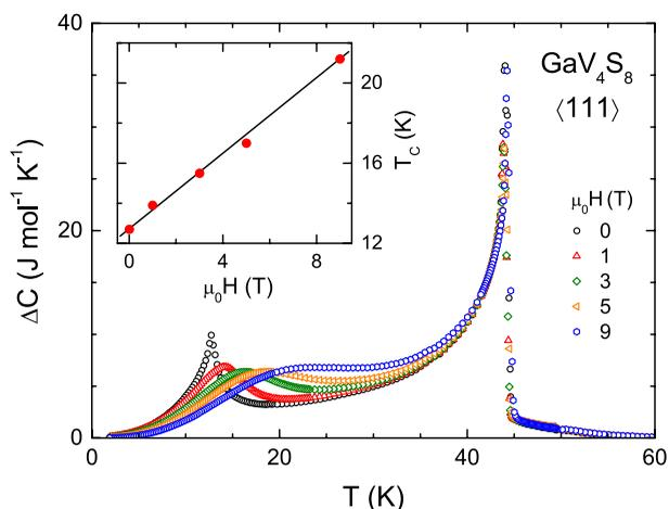
**Figure 4.** (colour online) Magnetic-field dependence of the heat capacity after subtracting the phonon contributions, which are indicated by the solid line in Figure 3. The excess heat-capacity  $\Delta C$  at magnetic fields between 0 and 9 T is plotted vs. temperature. The inset shows the dependence of the peak maximum of the magnetic anomaly vs. the external magnetic field. The solid line is drawn to guide the eye.
