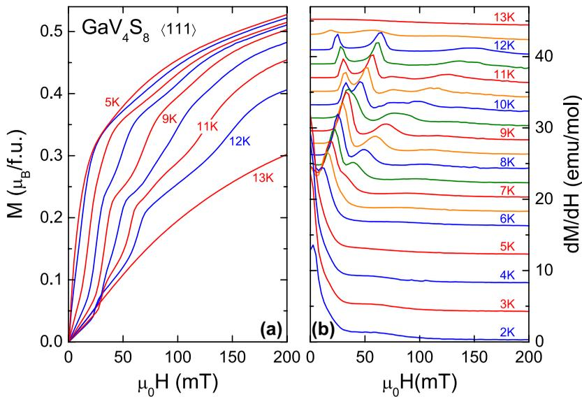
**Figure 7.** (colour online) (a) Low-temperature magnetisation of GaV<sub>4</sub>S<sub>8</sub> as measured in external magnetic fields along the <111> direction and between 0 and 200 mT for a series of temperatures between 5 and 13 K. (b) Derivative of the magnetisation for external magnetic fields between 0 and 200 mT and temperatures between 2 and 13 K. For clarity, the absolute values of the derivatives have been shifted along the vertical axis.
