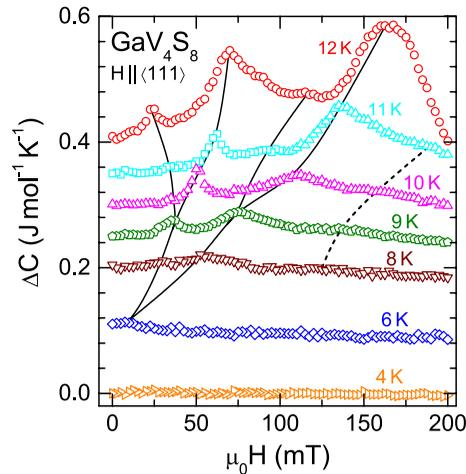
**Figure 9.** (colour online) Results of magnetocaloric experiments on GaV<sub>4</sub>S<sub>8</sub> with the external magnetic field applied along the  $\langle 111 \rangle$  direction: Excess-heat capacity as function of the external magnetic field between 0 and 200 mT for a series of temperatures between 4 and 12 K. For clarity reasons, data for  $T > 4$  K are vertically shifted. Tentative phase boundaries are indicated by solid and dashed lines.
