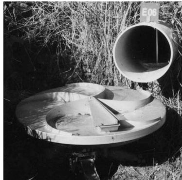
Figure 3.3. Coshocton-type wheel runoff sampler at the Scheyern Experimental Farm.
