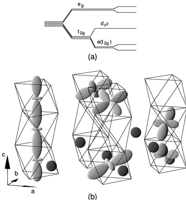
FIG. 4. (a) Crystal-field splitting of the vanadium  $3d$  levels due to the symmetry reduction from octahedral  $\rightarrow$  trigonal (distortion along the  $c$  direction)  $\rightarrow$  orthorhombic (zig-zag chain developed below  $T_S$ ). (b) Perspective view of the crystal structure of  $\text{BaVS}_3$ . The orientation of the low-lying orbitals derived from  $t_{2g}$  is also displayed.
