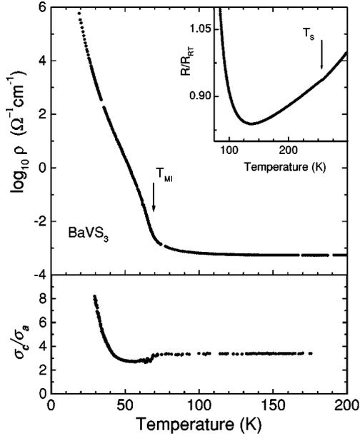
FIG. 1. Temperature dependence of the resistivity  $\rho_c(T)$ , and the conduction anisotropy  $\sigma_c/\sigma_a$  in  $\text{BaVS}_3$ . The arrows indicate  $T_S$ ,  $T_{MI}$ , and  $T_X$ , respectively.
