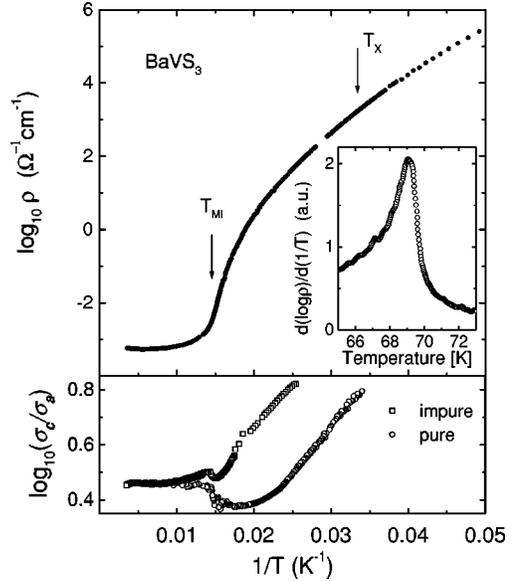
FIG. 2. Arrhenius plot of the resistivity and the conduction anisotropy. The latter is shown for two crystals of different purity. Inset: the peak of  $d \ln \rho / d(1/T)$  defines  $T_{MI}$ .
