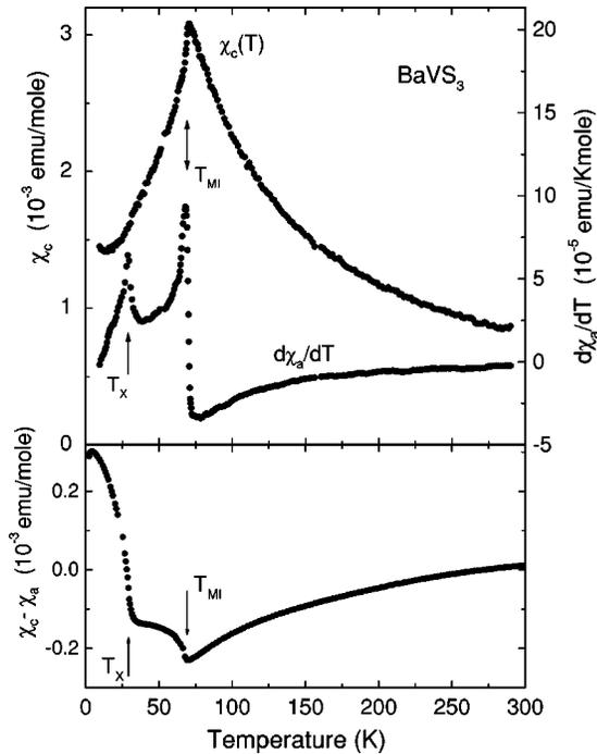
FIG. 3. Temperature dependence of the  $c$ -axis magnetic susceptibility  $\chi_c$ , the derivative of the  $a$ -axis susceptibility  $d\chi_a/dT$ , and the susceptibility anisotropy,  $\chi_c - \chi_a$ .
