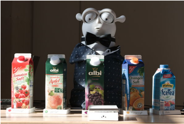
Figure 6: Prototype setup at the exhibition with Reeti robot, vessels, vessel holders and smartscale (front).
