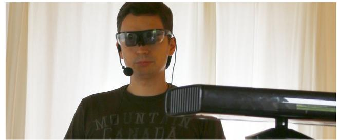
Figure 4. System setup: user wearing the HMD and microphone (far plane), and a Microsoft Kinect oriented towards him (near plane).
