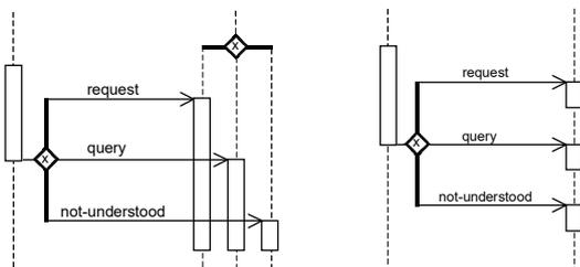
Figure 3. Full and abbreviated notation of XOR connection
