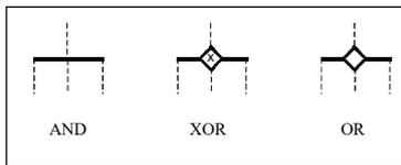
Figure 2. Connector types
