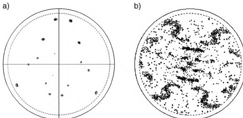
Fig. 4. Pole figure of LCMO deposited on 128°-rot LiNbO<sub>3</sub> (a) and YZ-cut LiNbO<sub>3</sub> (b). One clearly sees a higher degree of orientation in the case of 128°-rot LiNbO<sub>3</sub>.
