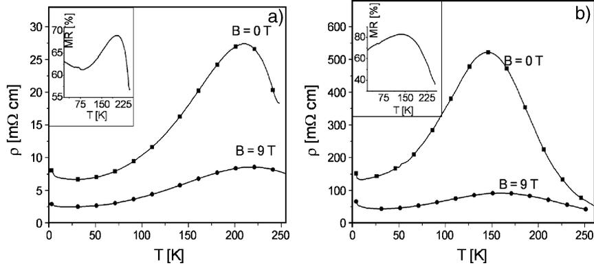
Fig. 5. Resistivity vs. temperature at  $B=0$  T (squares) and  $B=9$  T (circles). In the inset the magneto resistance  $MR = (\rho[0\text{ T}] - \rho[9\text{ T}]) / \rho[0\text{ T}]$  vs. temperature is shown. a) on 128°-rot LNB; b) on YZ-cut LNB.
