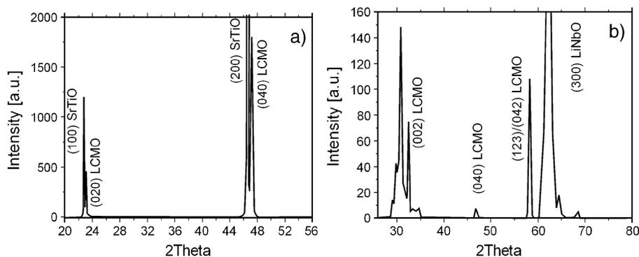
Fig. 3. Theta/2Theta scan of LCMO deposited on SrTiO<sub>3</sub> and YZ-cut LiNbO<sub>3</sub>.
