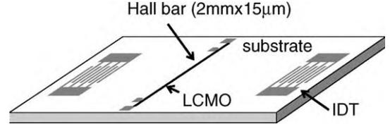
Fig. 1. Chip-design with two IDTs and LCMO hall-bar used for DC and SAW measurements. The thin Hall bar like LCMO stripe in the center of the SAW delay line is the sample under investigation.
