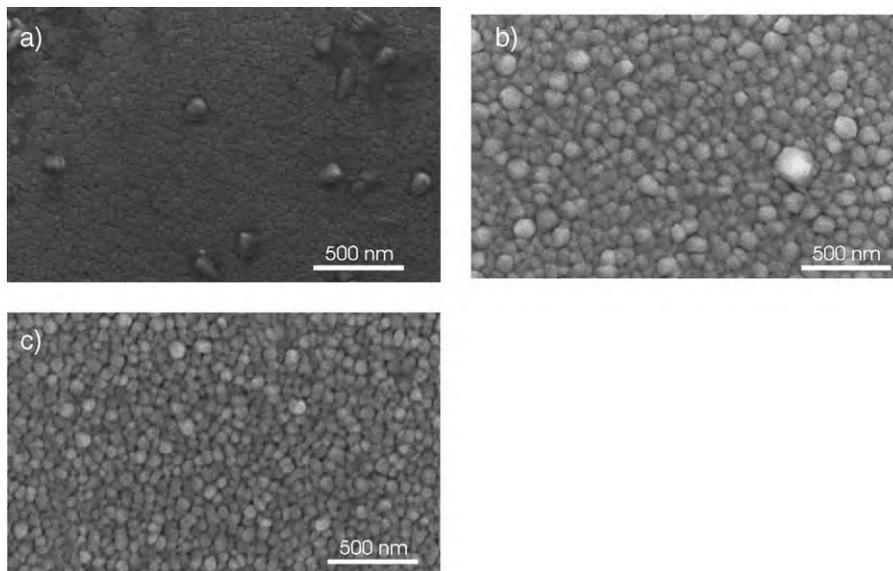
Fig. 2. SEM images of a LCMO film deposited on SrTiO<sub>3</sub> (a), 128° cut LiNbO<sub>3</sub> (b) and YZ-cut LiNbO<sub>3</sub>. The influence of the substrate on the film quality is clearly seen.
