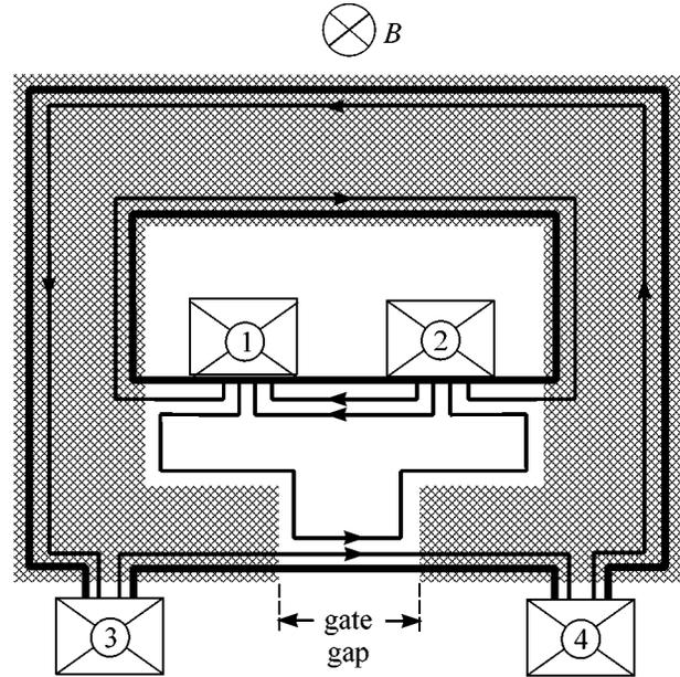
**Fig. 2.** Schematic diagram of the pseudo-Corbino geometry. Contacts are positioned along the etched edges of the ring-shaped mesa (thick outline). The shaded area represents the Schottky gate. Arrows indicate the direction of electron drift in the edge channels for filling factors of  $\nu = 2$  in the ungated regions and  $g = 1$  under the gate.
