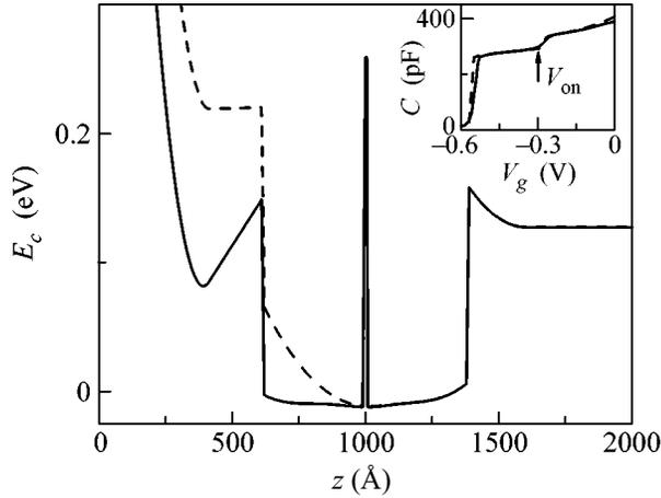
**Fig. 1.** Quantum well subband diagram at zero gate voltage (solid line) and at twice smaller electron conservation (dashed line) as calculated from the growth sequence of the structure (calculated using Poisson–Schrodinger solver by G. Snider). Inset shows the capacitance of the sample in dependence on the gate voltage calculated from the subband diagram (dashed) and measured in the experiment (solid). The magnetic field is zero.
