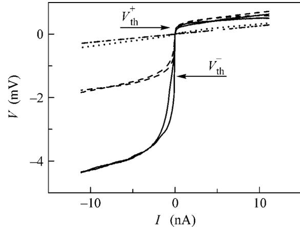
**Fig. 3.**  $I$ - $V$  curves for a total filling factor of  $\nu = 2$  and  $g = 1$  under the gate at different tilt angles. They are  $\theta = 0$  (solid line),  $\theta = 30^\circ$  (dashed line),  $\theta = 45^\circ$  (dotted line). Dash-dot line depicts fully equilibrium  $I$ - $V$  curve, calculated from Landau-Buttiker formulas. The normal magnetic field is constant and equals 8.7 T.
