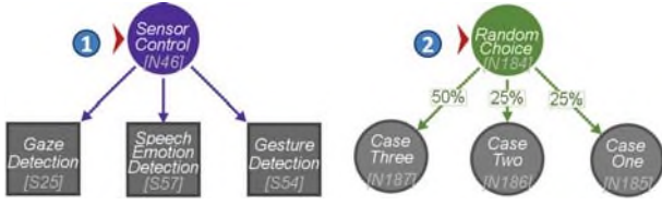
Figure 5: ① Concurrent processes with fork edges. ② Randomization with multiple probability edges.
