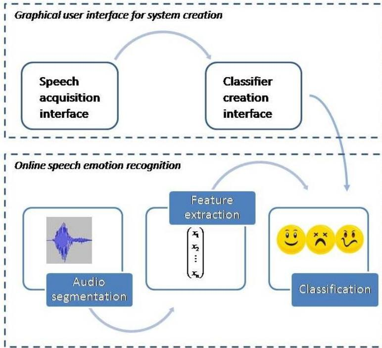
**Fig. 1.** Overview of the two modules of EmoVoice: The graphical user interface allows for convenient speech corpus and classifier creation. The online recognition module can be plugged into other applications and continuously tracks the emotional state of the user as expressed in his/her voice.
