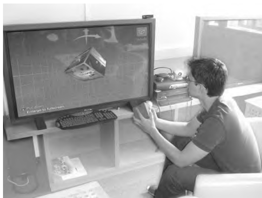
Figure 1: A user is interacting with the cube to control the TV-channels on the screen.
