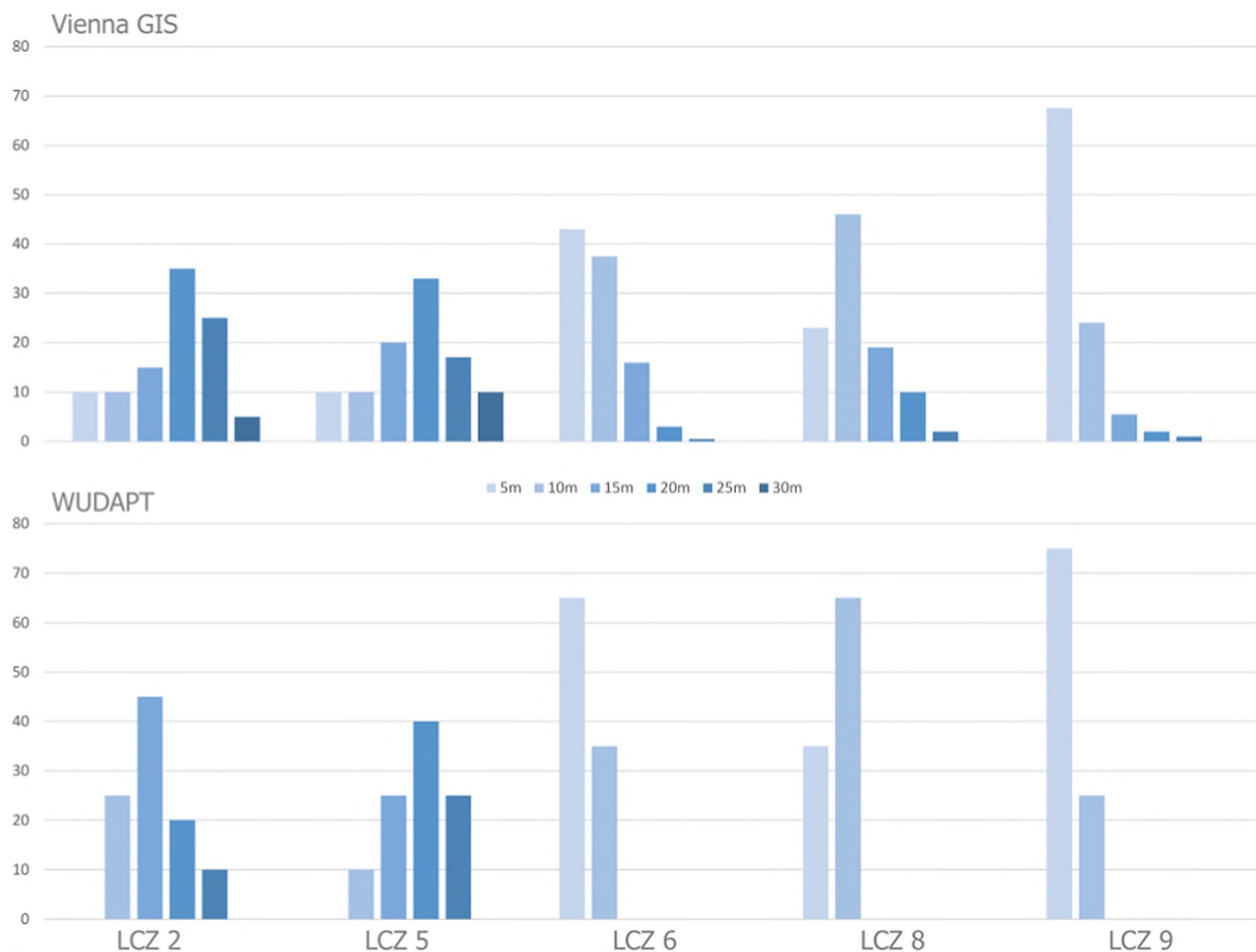
Fig. 17. Different LCZ morphological parameterisations of the city of Vienna, Austria in the BEP-BEM model, embedded in the WRF climate model, by source of parameters. A detailed building parameter GIS dataset is used for Vienna GIS and LCZs' ranges of parameters are used for WUDAPT. In the Vienna GIS case, heights are aggregated to 5 m intervals (the 5 m value represents heights from 0 to 5 m, etc.). See Hammerberg et al. (2018) for details.
