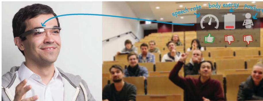
Figure 2. The Logue social augmentation system delivers live visual feedback to a person speaking in public via a head-mounted display.
