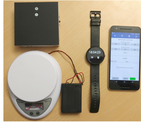
Figure 3: All devices used for the high fidelity system prototype: the two Bluetooth scales, a Moto 360 smartwatch and a Nexus 6P smartphone)
