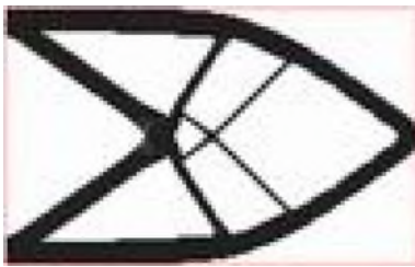
Fig. 1 Topology optimization of a cantilever
