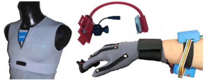
Figure 2: Newly developed wearable sensor devices. From left to right: e-Shirt, eye tracker and glove.
