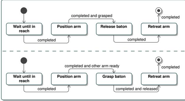
Figure 5: State machine: Robot interaction, adapted from [2]
