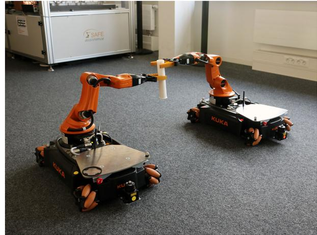
Figure 1: Robots handing over a baton, adapted from [2]
