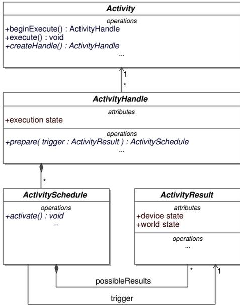
Figure 2: Relevant classes for task definition and execution
