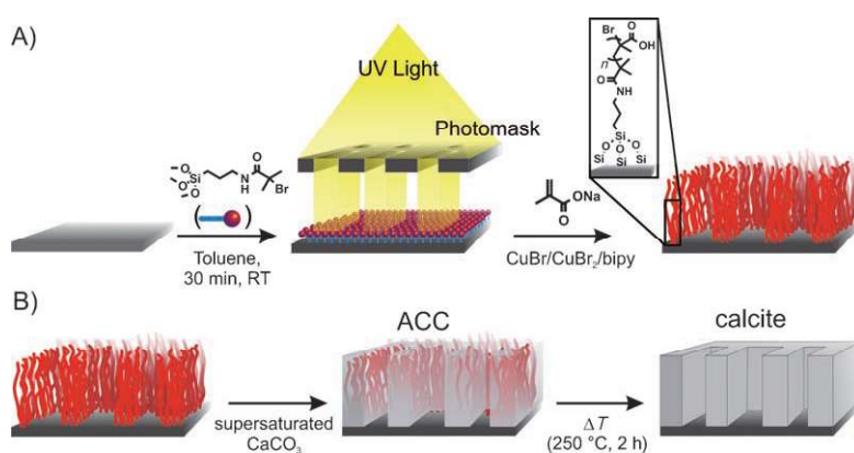
Figure 1. Fabrication of microstructured calcite films. A) Synthesis of PMAA brushes by SI-ATRP of sodium methacrylate from photolithographically patterned ATRP initiator functionalized substrates (bipy=2,2'-bipyridine). B) Directed deposition of a thin, metastable layer of amorphous calcium carbonate (ACC) and subsequent temperature-induced transformation of the metastable ACC layer into a microstructured, polycrystalline calcite film.
