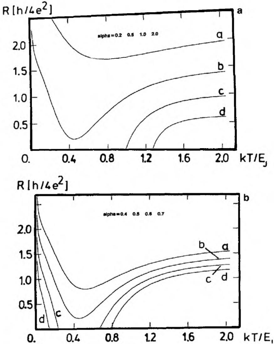
Fig. 4. (a) Temperature dependence of the resistivity, measured in units of  $h/4e^2 R_n$ , for  $E_J/E_C = 0.4$  and different values of  $\alpha$ : (a)  $\alpha = 0.2$ ; (b)  $\alpha = 0.5$ ; (c)  $\alpha = 1.0$ ; (d)  $\alpha = 2.0$ . (b) Same as in (a) for different values of  $\alpha$ : (a)  $\alpha = 0.4$ ; (b)  $\alpha = 0.5$ ; (c)  $\alpha = 0.6$ ; (d)  $\alpha = 0.7$ .
