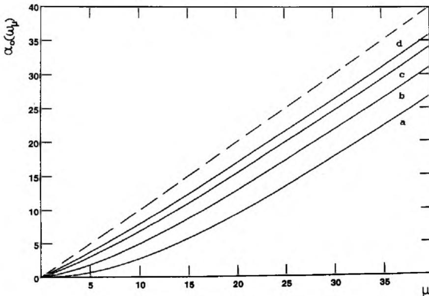
Fig. 1. Plotted is the quasiparticle damping kernel  $\alpha_{qp}(\omega_\mu) = -(1/2e^2 R_n)2\pi kT\alpha_0(\omega_\mu)$  as a function of  $\mu = \hbar\omega_\mu/2\pi kT$  for  $\Delta/\pi kT = 20$ , and different (fixed) values of  $\Gamma_0 = \Gamma/\pi kT$ : (a)  $\Gamma_0 = 0$ ; (b)  $\Gamma_0 = 10$ ; (c)  $\Gamma_0 = 20$ ; (d)  $\Gamma_0 = 30$ . The dashed line is the Ohmic result  $\alpha_0 = \hbar|\omega_\mu|/2\pi kT$ .
