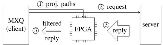
Fig. 4. *MXQuery/H* system design. For each query, *MXQuery/H* sends projection path information to the FPGA ① and a data request to the server ②. Data is sent back and filtered on the FPGA ③. All communication is through an Ethernet network.
