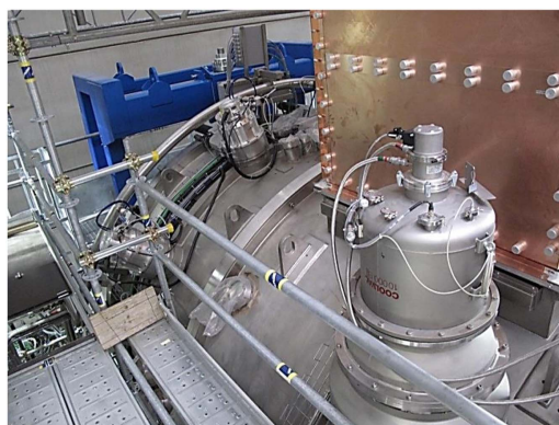
Figure 23. View of turbomolecular and cryogenic pumps installed around the SPIDER Vacuum Vessel.
