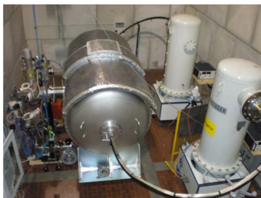
Figure 24. View of the HVPTF 800 kV setup. The tank with the lead screening on the top and the two \pm 400 kV/1 mA power supplies are shown. Connection to the electrodes is made via coaxial XLPE cables.
