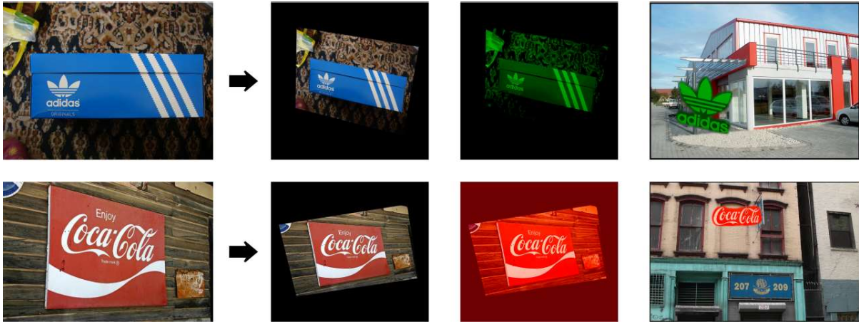
Figure 2: Two examples of synthetically generated images. Starting from a base image, a random perspective transform is applied, followed by gaussian blur (not shown), color augmentation (exaggerated for viewing purposes) and background replacement.
