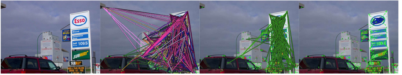
Figure 6: Example detection of the Esso logo: Original image (left), all detected edges of any class (middle left), edges belonging to real class (middle right) and the final detected triangles (right)
